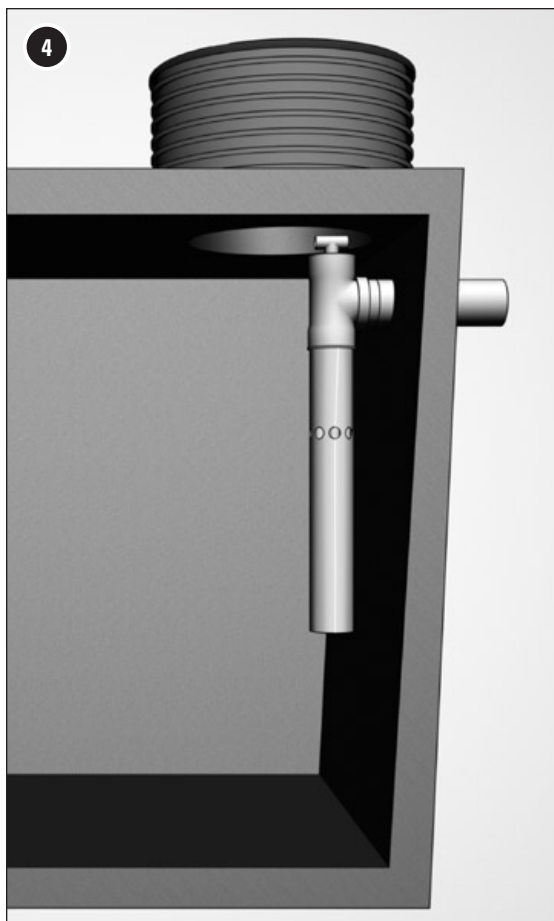
Orenco® effluent filter installed on the septic tank outlet.
