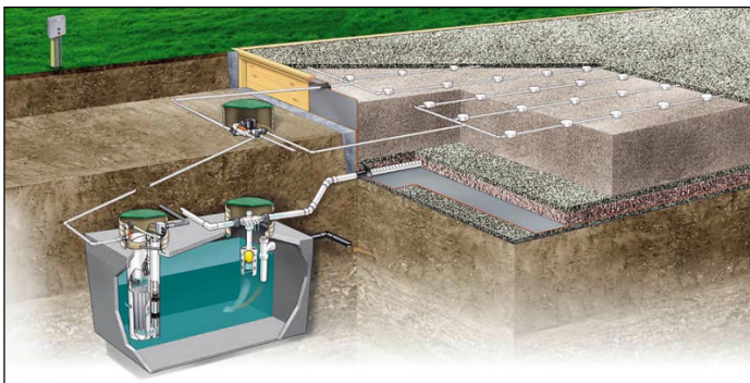
Figure 2: Recirculating sand filter (RSF)
